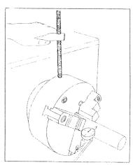
CAUTION: Never use more than hand pressure with the wrench furnished to tighten pinion or adjusting screws or you will destroy the precision of the chuck
